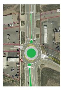
**Two Lane N-S Alternative -** Recommended. Capacity analyses reveal the 2X1 lane roundabout is the correct design. (A 150-foot diameter 2X1-lane concept is depicted here.)
