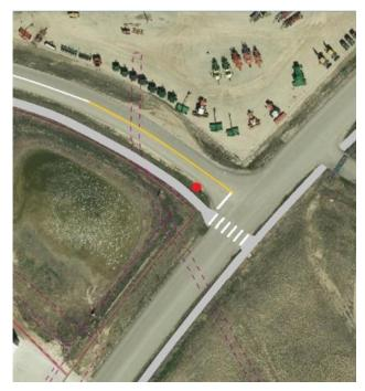
At the US-20/26 / Blackmore Road intersection, the study recommends improved signs, markings, and intersection lighting, and consideration of a speed reduction from 55 to 40 MPH and a pedestrian crossing. Long term, the corridor may be considered for signalization and retrofit as an "urban boulevard" using indirect left turns for access management and safety improvement.
