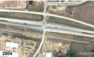
The two-way Average Daily Traffic (ADT) on US-20/26 in the year 2020 is 5,300 ADT, down from a peak of 6,000 ADT in 2015. The current Blackmore Road traffic volume is about 900 vehicles. Crash records from 2015 to 2019 show a pattern of two angle crashes, three rear end crashes, and three loss of control crashes; all involving the south leg of the intersection. There were three injury crashes resulting in four injuries during the study period.
